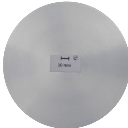
Macrosection, d178 mm: Segregation 2,9 mm
