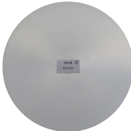
Macrosection, d252 mm: Segregation 5,5 mm
