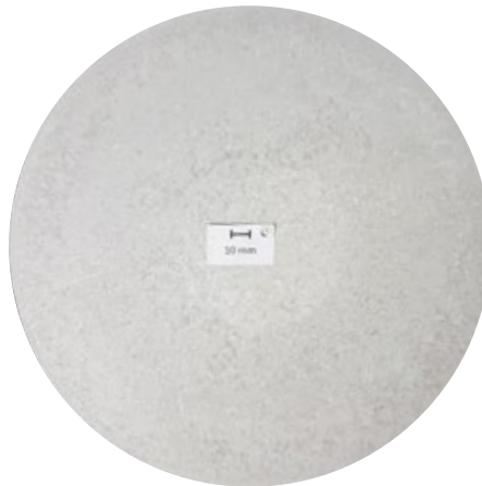
Macrosection, d278 mm: Segregation 2,1 mm
