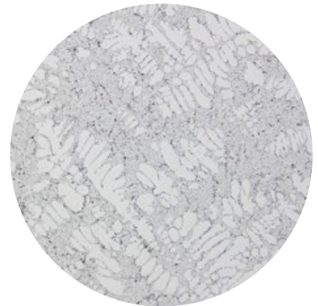
Microsection, d278 mm (25 times magnification)
