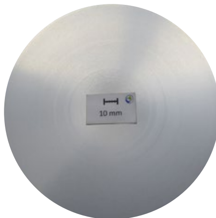
Macrosection, d178 mm: Segregation 2,7 mm
