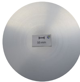
Macrosection, d178 mm: Segregation zone 2,7 mm
