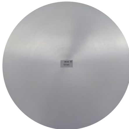
Macrosection, d424 mm: Segregation 8 mm
