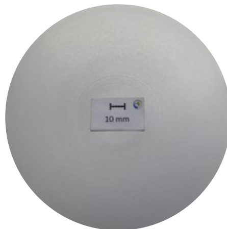
Macrosection, d177 mm: Segregation zone 3,1 mm
